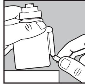
4. Break the seal on the vent tube to allow air flow. Tab can be completely removed or bent enough to open vent and remain attached.
